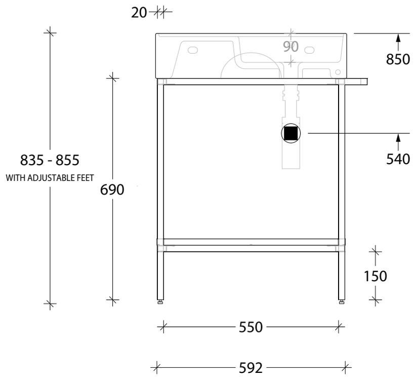
RECOMMENDED ROUGH IN SPECS FOR PLUMBER BASED ON INSTALLED BENCH HEIGHT (850) WITH ADP SUBWAY BOTTLE TRAP
