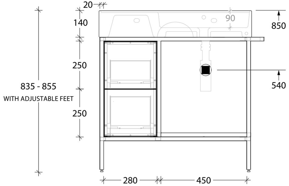
RECOMMENDED ROUGH IN SPECS FOR PLUMBER BASED ON INSTALLED BENCH HEIGHT (850) WITH ADP SUBWAY BOTTLE TRAP
