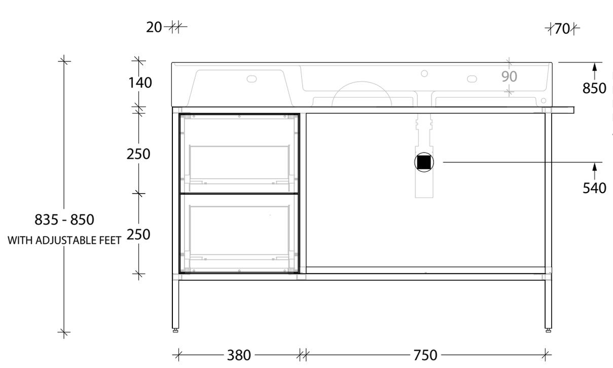
RECOMMENDED ROUGH IN SPECS FOR PLUMBER BASED ON INSTALLED BENCH HEIGHT (850) WITH ADP SUBWAY BOTTLE TRAP
