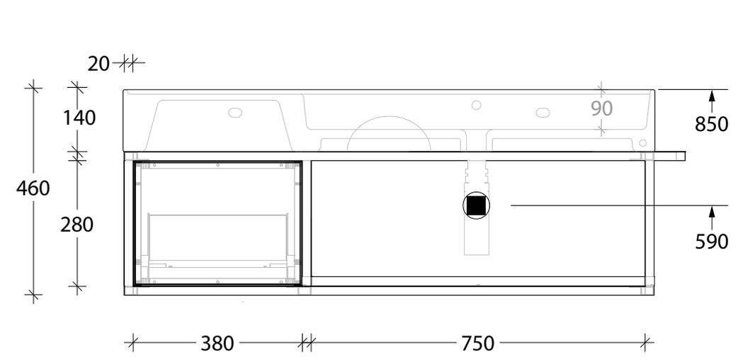
RECOMMENDED ROUGH IN SPECS FOR PLUMBER BASED ON INSTALLED BENCH HEIGHT (850) WITH ADP SUBWAY BOTTLE TRAP
