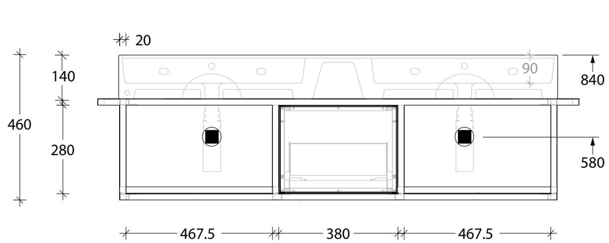
RECOMMENDED ROUGH IN SPECS FOR PLUMBER BASED ON INSTALLED BENCH HEIGHT (850) WITH ADP SUBWAY BOTTLE TRAP
