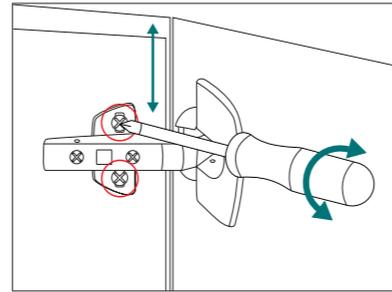
Loosen the top and bottom screw on mount plate, adjust door height by moving door up or down, then retighten screws.
