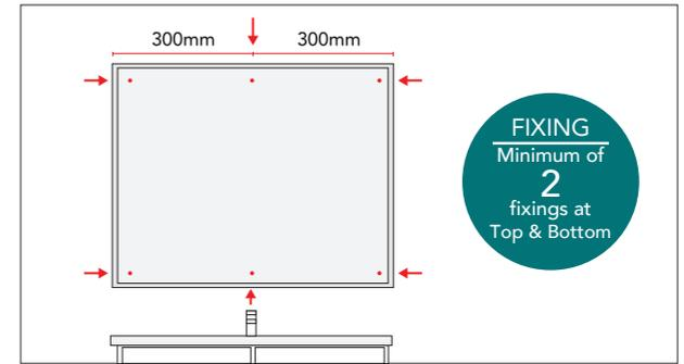
Securely fasten cabinet to the wall through back with appropriate screws/bolts at TOP and BOTTOM of cabinet. Evenly space apart the horizontal fixings at a maximum of 300mm apart.
