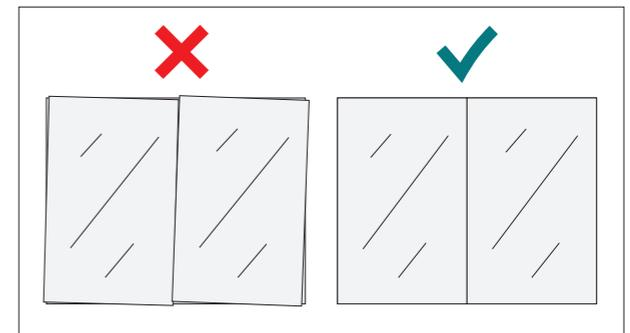
Install doors back onto cabinet and make adjustments to align the doors correctly. See opposite page for instructions.
