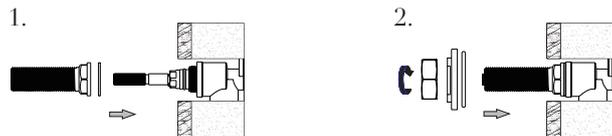
1. Screw Ceramic Spindle (10) into wall body. Insert Fibre Washer (9) and Spindle Lock Nut (8). Fasten.
