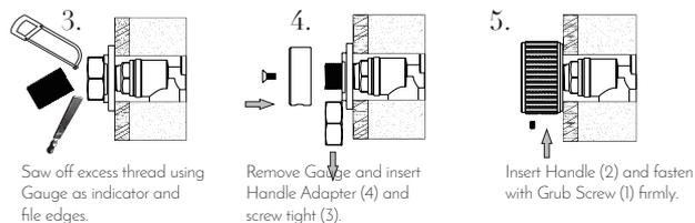
3. Saw off excess thread using Gauge as indicator and file edges.
