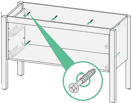
Securely fasten the vanity to the wall through back of vanity with appropriate screws/bolts at TOP and BOTTOM of cabinet. Fix the cabinet through the top left and right hand brackets and evenly space apart the horizontal fixings at a maximum of 300mm apart. For the bottom start the fixing points no further than 100mm from each end of the cabinet and no higher than 50mm from the base panel.
