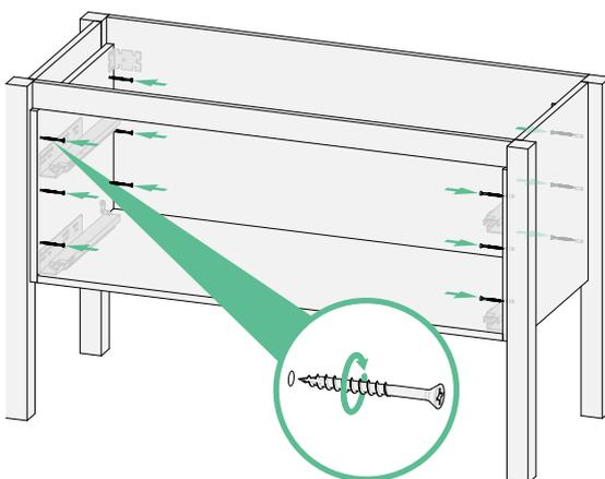
Using the provided 40mm Hospa screws, screw through the holes in the vanity ends, into the legs to secure into place.
