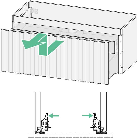
Remove all drawers from vanity by squeezing both levers in on the underside of the drawer, at the same time (to activate release) and pull drawer out to remove.
