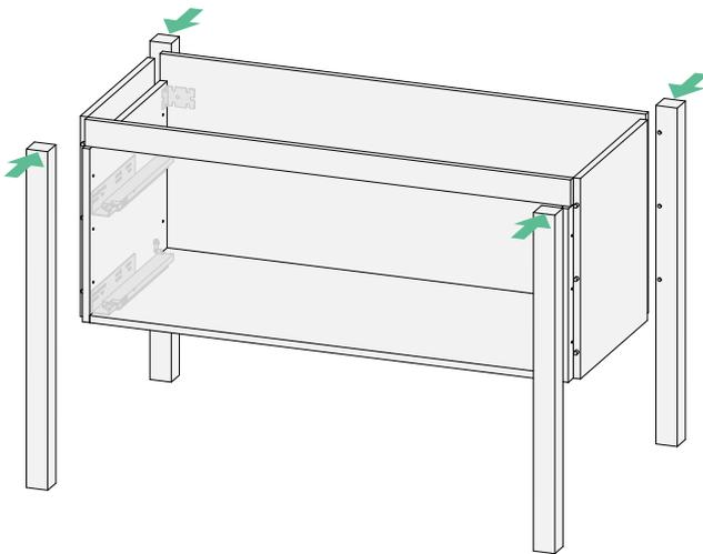
Align the legs with the dowels in the vanity end panels and lightly tap them into place ensuring a snug fit.
