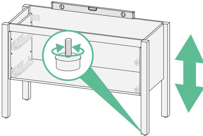
Align vanity to wall and use the adjustable feet to level, using a spirit level to ensure levelling is correct.
