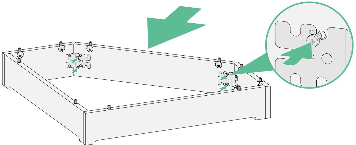
Align the front kickboard piece with the assembly and connect using the provided screws through the bracket slots.
