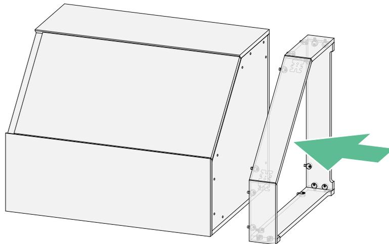
Carefully tip cabinet on its back and align the kickboard using the drill holes in the cabinet base. Push fit kick assembly and turn cam screws to lock the kickboard in place.
