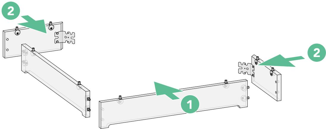
Connect side and back toes of kickboard by aligning cams with their respective sockets and turn phillips head screw in cam clockwise to lock part in place.
